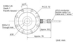
\* Connector can be attached to the cable according to your requests Refer to 84 pages for details
